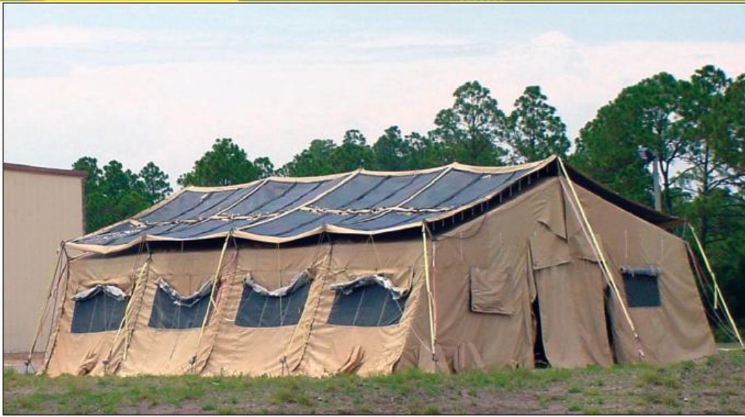
Figure 2. Flexible solar cell technology incorporated into a military tent
